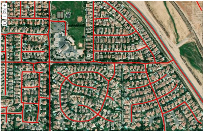
Fig 2. Roads detected using deep learning and converted to geographical features
