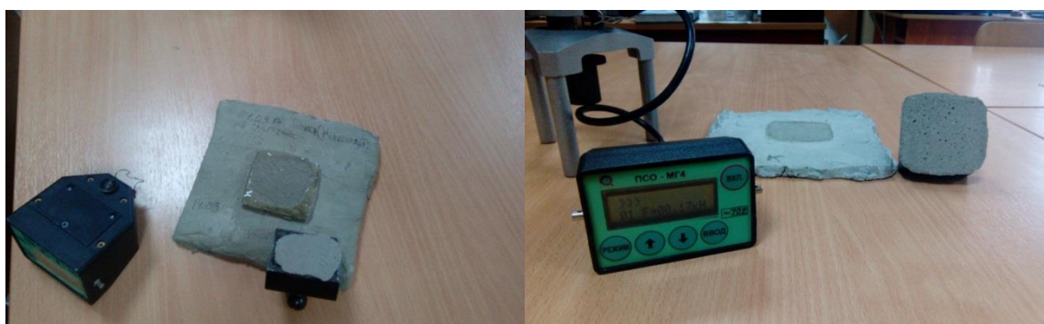
Fig. 2. Tests of the adhesive strength of a polymer-cement composite (a) and a control sand-cement sample (b)
