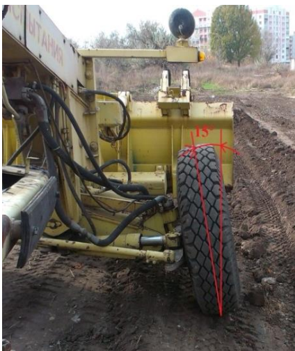
Figure 4. Adjustment of a wheel leaning angle
