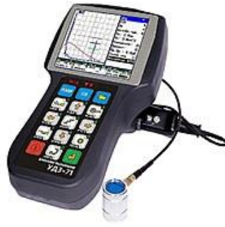
Fig. 4. UD-3-71 (Ultrasonic General-Purpose Flaw Detector)
