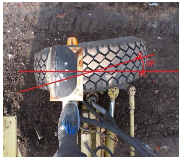
Figure 5. Adjustment of a wheel turning angle
